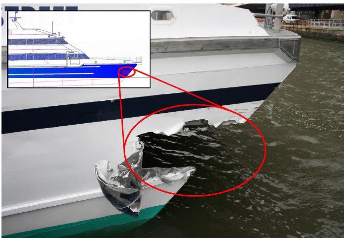
Fig. 2 – Damage to Seastreak Wallstreet, Source: NTSB Accident report
